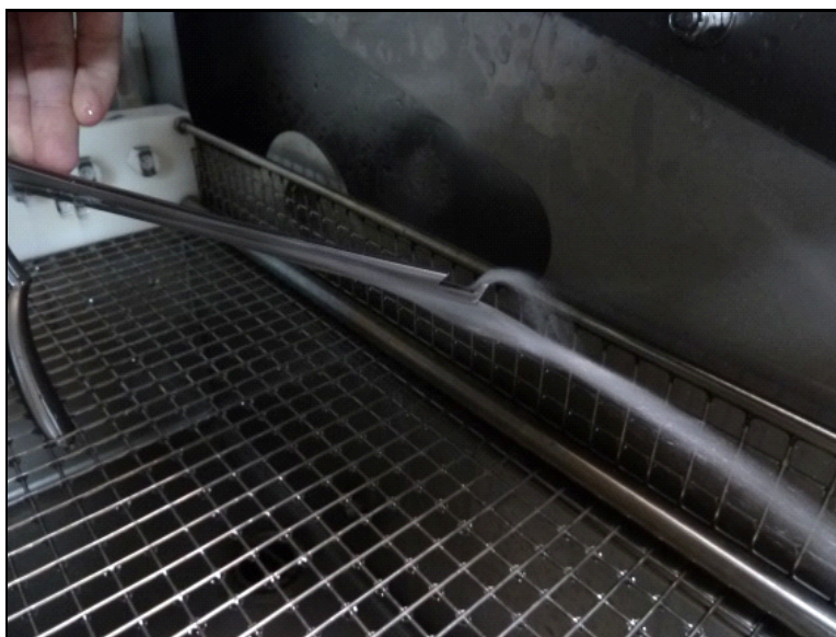
Elmed's Clear Flush® Kerrison Being Flushed with an Enzymatic Detergent in an Automatic Washer.
